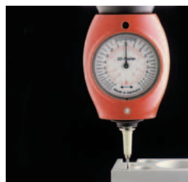
2. Zero position has been reached. The effective total length of 3D-Taster has been preset; the NC-control can be set to "Zaro".
