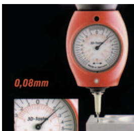
1. The stylus touches the workpiece surface. The difference value can be read (example:0,08mm).
