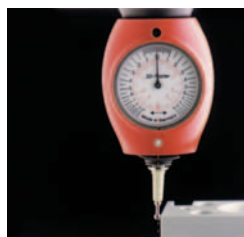
2.Zero position has been reached, spindle axis= workpiece edge: The NC-control can be set to "Zero"
