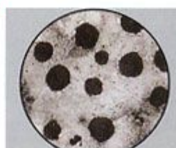
Microphotograph for ductile cast iron
